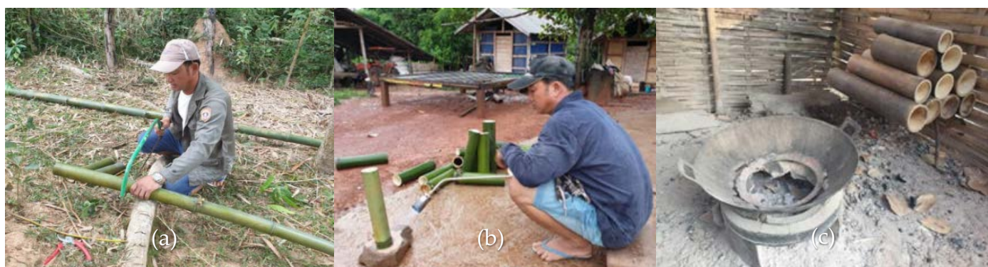
Figure 6. Bamboo harvesting, collection, and management steps: (a) cutting bamboo culm by node, (b) treating bamboo outer skin with gas torch, and (c) drying the treated bamboo material using a kitchen stove.
