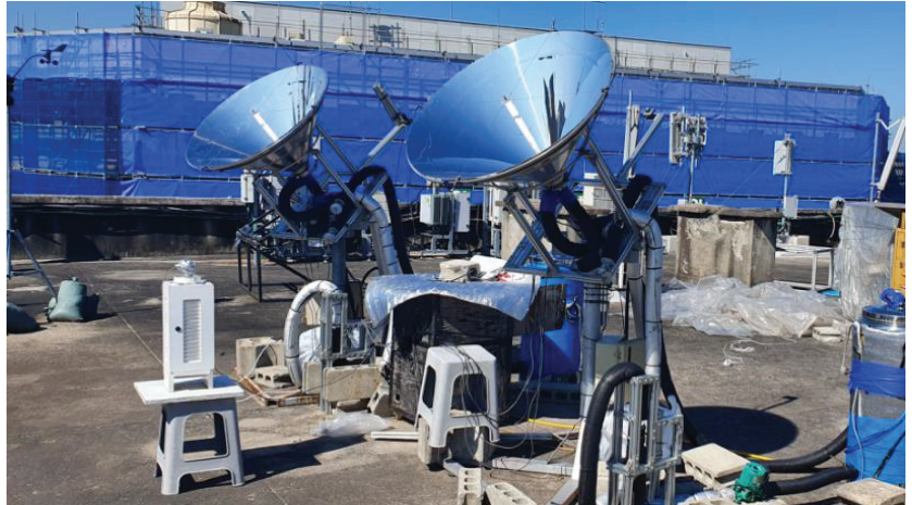
Figure 1. Experimental setup of the conical solar collector system.
