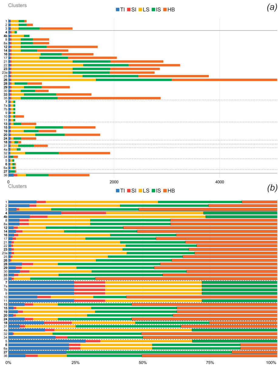
Figure 5. Ladder diagrams showing contributions to structural complexity (bits per unit cell) (a) and normalized contributions (in %) (b) for the structures based on uranyl carbonate finite clusters. Legend: TI = topological information; SI = structural information; LS = layer stacking; IS = interstitial structure; HB = hydrogen bonding. See Table 2 and text for details.
