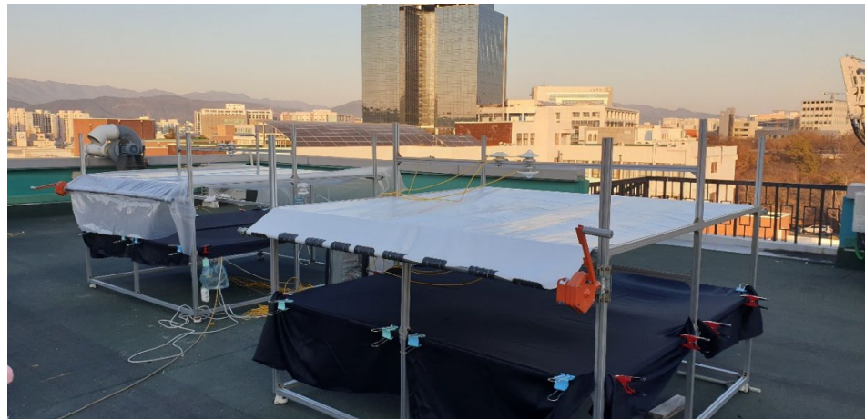
Figure 8. Experimental setup for determining the radiometric properties of the greenhouse materials.
