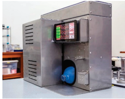
Figure A2. Mechanical ventilation system OxygenIPPE, where the novel air low sensor/transducer is implemented.
