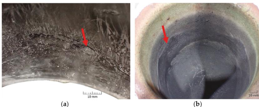
**Figure 14.** Visual appearance of the crucibles after the experiments: (a) traces of attack on the  $\text{Al}_2\text{O}_3$  crucible wall in Design 1; (b) appearance of the  $\text{MgO}$  crucible after experiment 2 with obvious adhesions.
