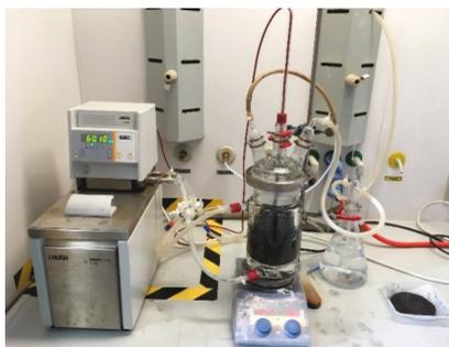
**Figure 4.** Setup of the leaching process under optimized conditions in the laboratory (double walled reaction vessel with a reaction volume of one liter and a thermostat to control the chosen process temperature).
