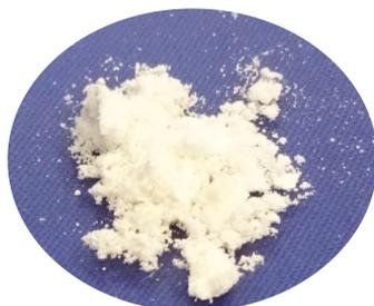
**Figure 8.**  $\text{Li}_2\text{CO}_3$  as a product after precipitation of  $\text{LiHCO}_3$  by heating up at 100 °C.
