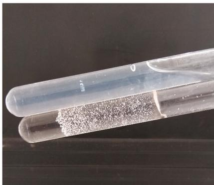
**Figure 14.** Solution before (top) and 30 min after addition of 17.9 M H<sub>2</sub>SO<sub>4</sub> (bottom).
