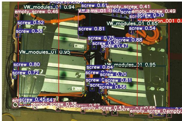
**Figure 9.** YOLOv3 output results: all screws, modules, transverse covers, and BMS are detected, classified, and localised.
