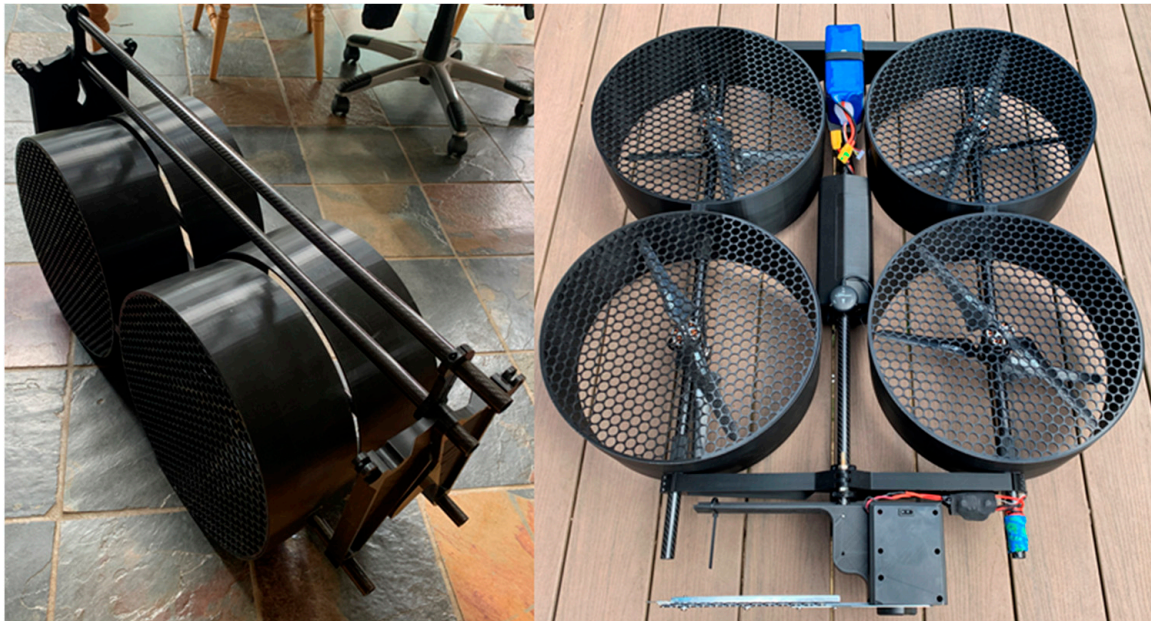
Figure 7. Version 3.0 protected the propellers with the use of 3D printed ducts. The design was capable of folding for ease of transport. The calculations used for estimating flight performance were found to be optimistic, with the system unable to fly out of ground effect.
