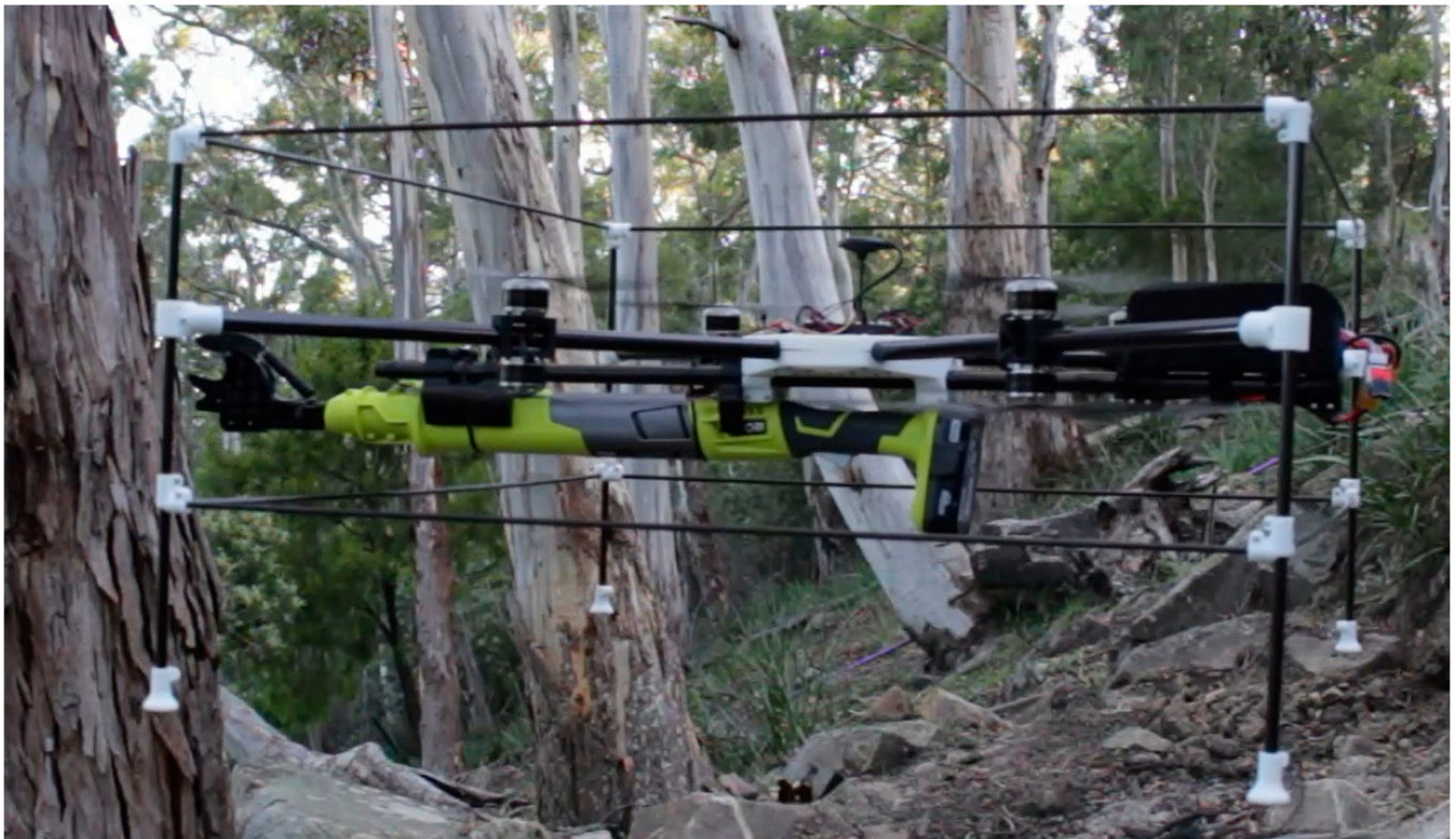
Figure 2. Version 1 was most similar to [39]. The first sampling approach used powered secateurs to drop branches of up to 30 mm in diameter to the ground for retrieval. This required precise aiming and flight control during cutting, and while it was functional, a more practical approach that required less precise flight control was sought.
