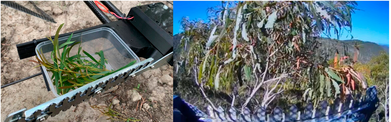
Figure 4. A single-handed hedge trimmer was modified and integrated into a custom 3D printed housing with a removable sample container. A manual safety switch is shown in the top-right of the left image, which allows the operator to prevent the tool from running unexpectedly. Right shows a camera view of the tool while in flight, about to collect a canopy sample.
