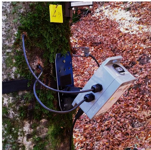
Figure 1. A beech tree monitored with a TreeTalker (power supply not shown).
