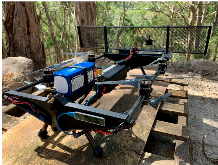
Figure 9. Visual Inertial Odometry (VIO) was used to provide precise flight control to Version 3.1 of the UAS. The VIO sensor was an Intel Realsense T265 and was soft mounted on the rear of the aircraft.
