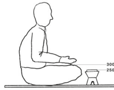
Figure 3. The difference between the height of a standard rehal and the height where the hands of an average adult male would rest.
