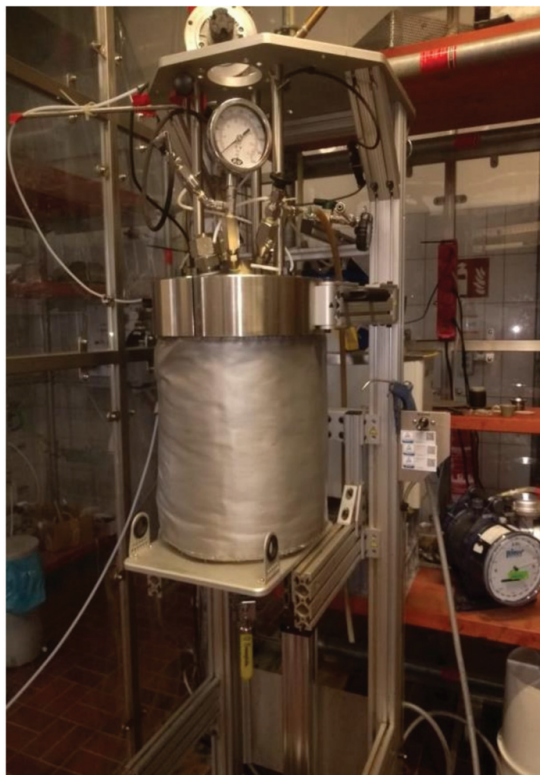
Figure 3. Pilot-scale stirred tank stainless steel reactor of 18.92 P L (Parr, USA, Model: 4555).
