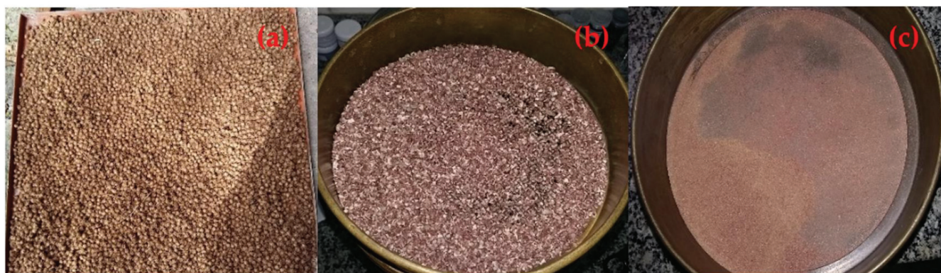
Figure 2. Material after drying, milling, and sieving process of Açai seeds (seeds + fibers (a); comminuted seeds + fibers (b); and sieved seeds (c)).
