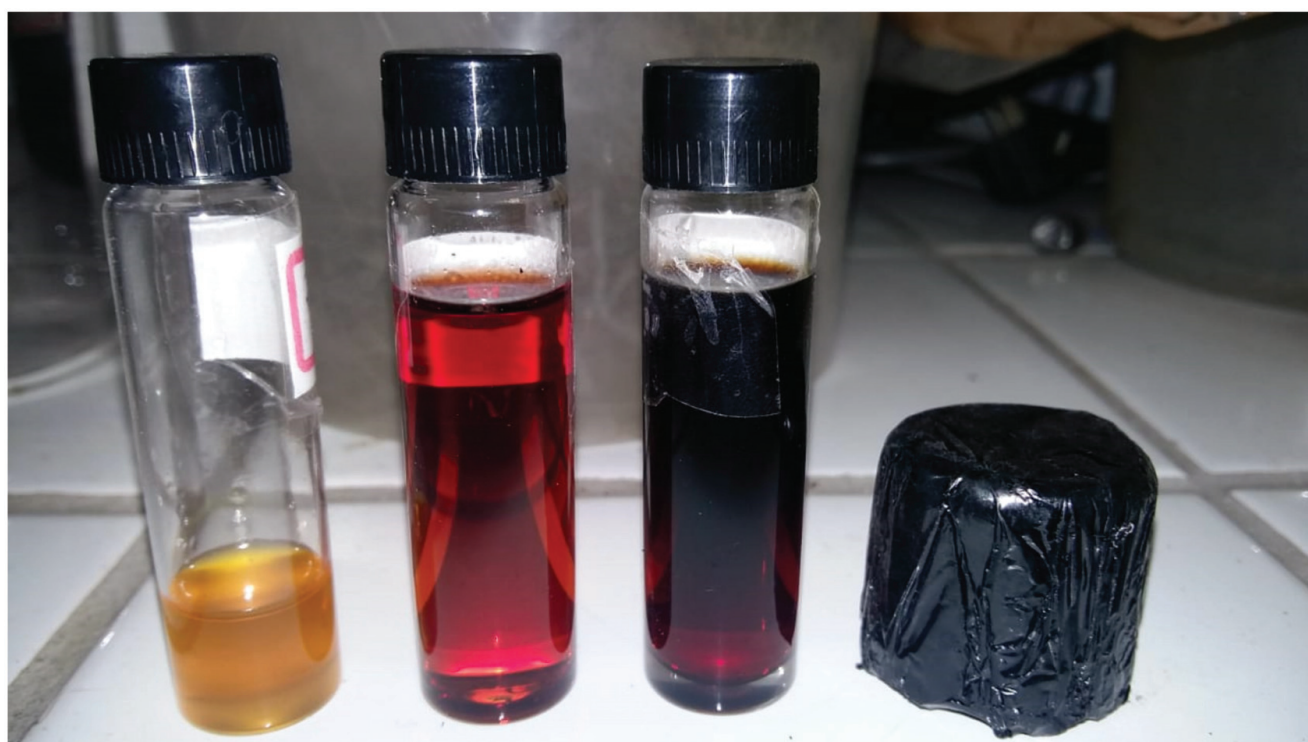
Figure 9. Distillation fractions [gasoline (yellow), light kerosene (red), and kerosene (red dark)-like boiling range temperature fossil fuels] and bottoms [Raffinate (black solid)] obtained by fractional distillation of bio-oil produced by pyrolysis of Açai ( Euterpe oleracea , Mart.) seeds at 450 °C and 1.0 atmosphere, in pilot scale.
