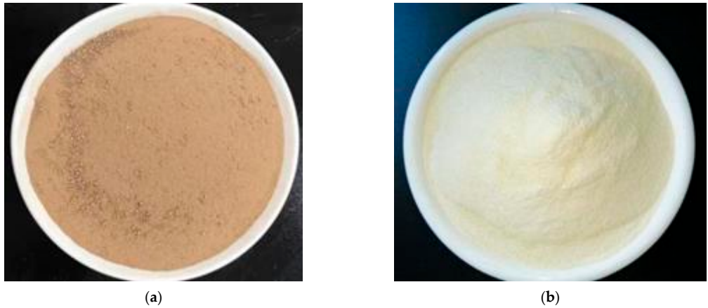
Figure 2. Samples of natural soil and xanthan gum: (a) silt; (b) xanthan gum.
