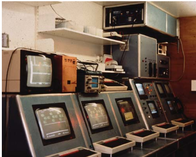
Figure 4. The Durham Mark III telescope control room. While the main DAQ was performed by a Motorola 68000 computer situated under the console, the system's interfaces were all BBC microcomputers. These were remarkable- and remarkably cheap-computers for their time. The copper box on top of the console contains the rubidium oscillator used for timing.
