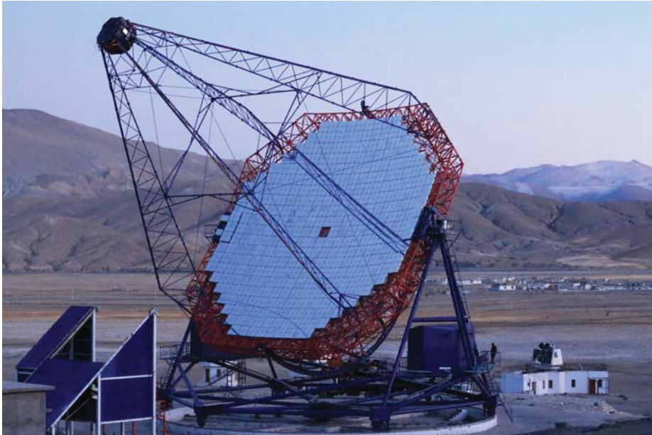
Figure 7. The 21 m diameter MACE \gamma -ray telescope at Hanle site (4270 m above sea level).
