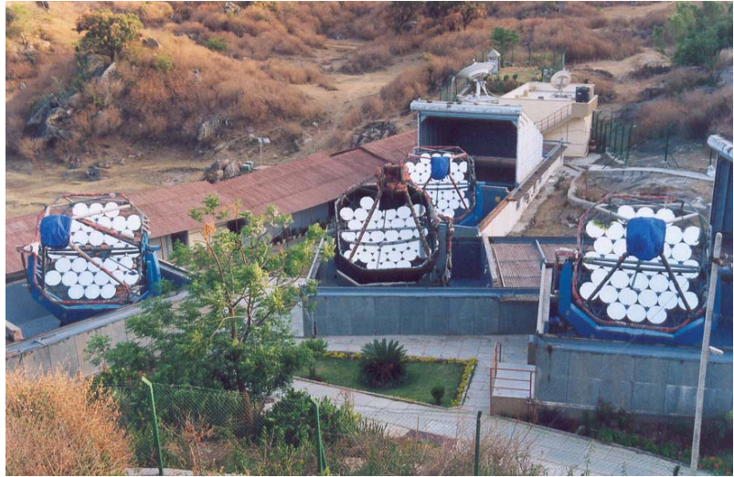
Figure 1. The TeV Atmospheric Cherenkov Telescope with Imaging Camera (TACTIC) telescope array operational since 2001 at Mount Abu, India. Single telescope at the center is being used as an imaging unit for TeV \gamma -ray observations.
