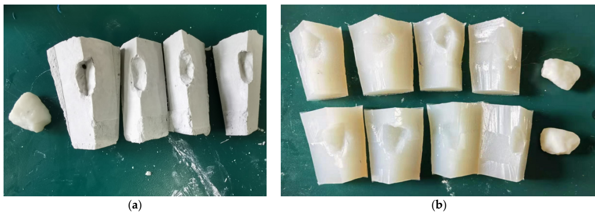
Figure 11. The prepared two molds (a): plaster mold; (b): silica mold.
