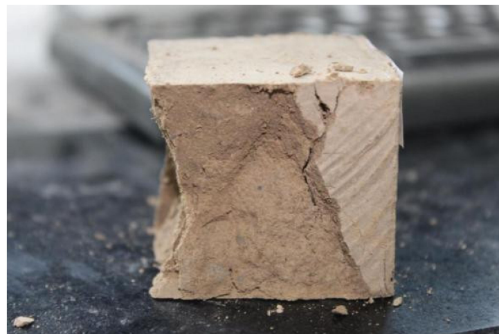
Figure 7. Fracture surface of conventional CSS sample.
