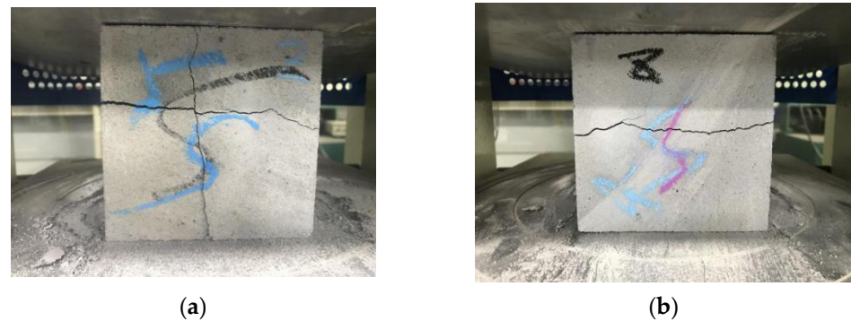
Figure 15. The printed cube sample cracks of (a) C plane and (b) reverse plane.
