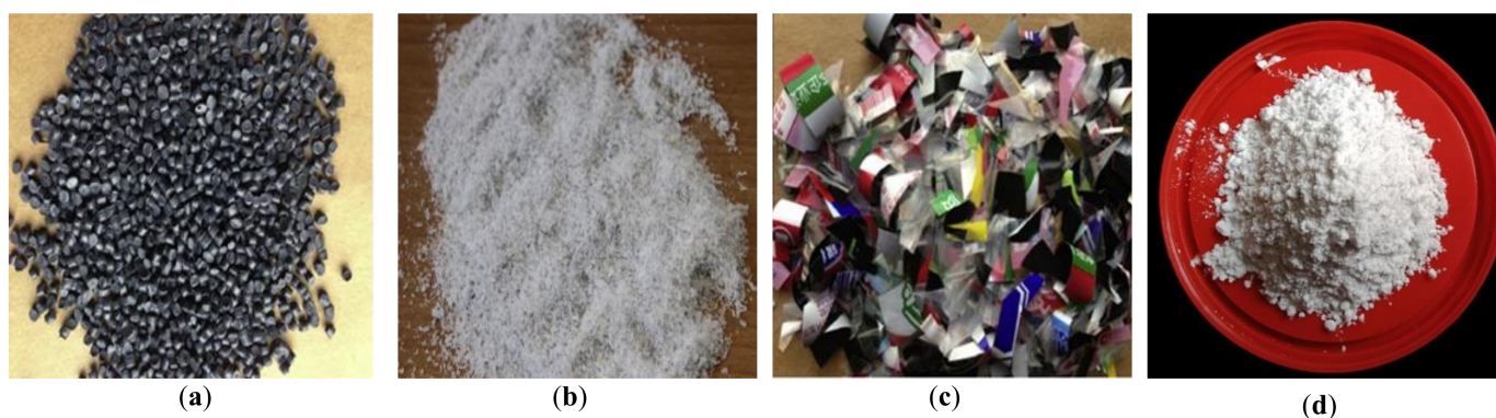
Figure 2. Various forms of waste plastics used as modifiers: (a) pellet [57]; (b) shredding [54]; (c) flake [57]; (d) powder [58]. Reprinted with permission from Refs. [54,57,58]. Copyright 2014 Elsevier publisher.
