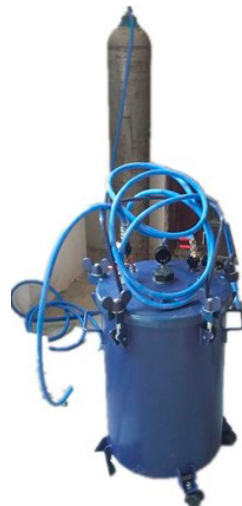
Figure 2. Apparatus of the accelerated carbonation test.
