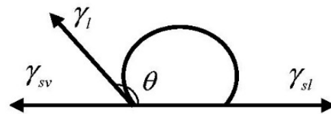
Figure 6. Schematic diagram of interface between the reagent and limestone.
