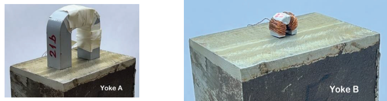
Figure 4. Photographs of two different size magnetizing yokes (Yoke A and Yoke B) on the top of the same block.
