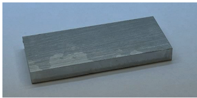
Figure 3. Photograph of the cladding itself (cut from the top of another cladded block).
