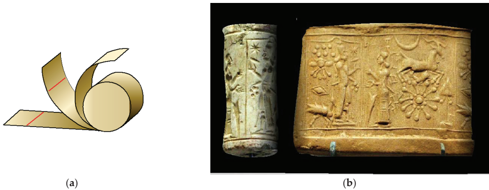
Figure 4. (a) An example of a developable surface, where a cylinder is unrolled into a plane. This surface is also ruled, and the pattern of parallel straight lines drawn on the cylinder surface is preserved during the transformation. Figure (b) shows an ancient Mesopotamian cylindrical seal (dating to about 5000 BC) and its imprint. [18].
