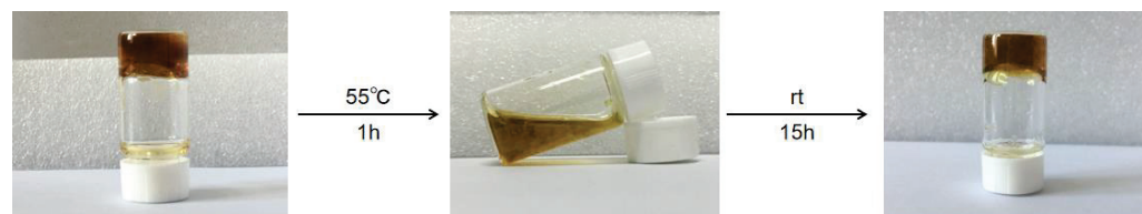
Figure 7. The gel–sol–gel transition cycle of H1 .
