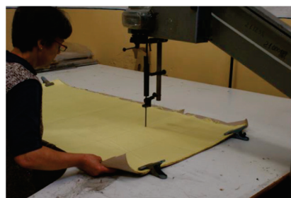
Figure 2. Cutting process of the layers for the ballistic package.
