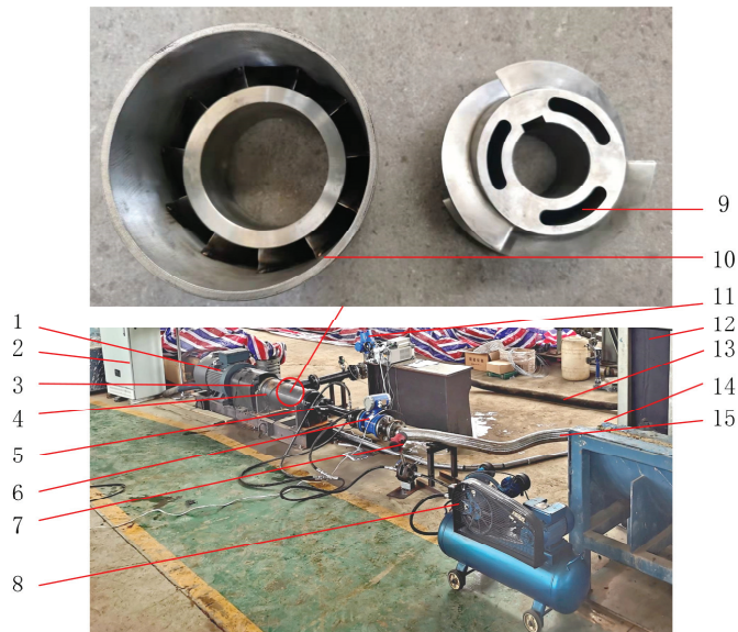
Figure 21. Experimental process diagram for the multiphase pump. (1) Motor; (2) frequency transformer; (3) torque and revolution speed sensor; (4) multiphase pump; (5) pressure sensor; (6) liquid flowmeter; (7) gas flowmeter; (8) air compressor; (9) guide vane; (10) impeller; (11) electronic throttle valve; (12) tank; (13) outlet pipe; (14) valve; (15) inlet pipe.
