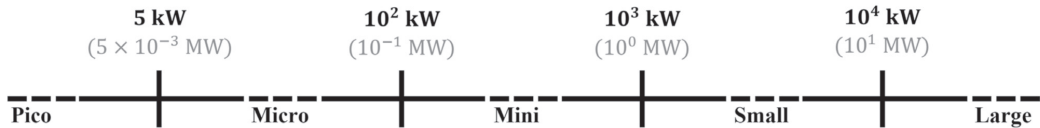
Figure 1. Classification of hydropower plants based on the installation capacity.
