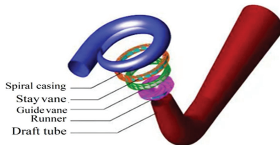
Figure 3. Model pump turbine calculation area.
