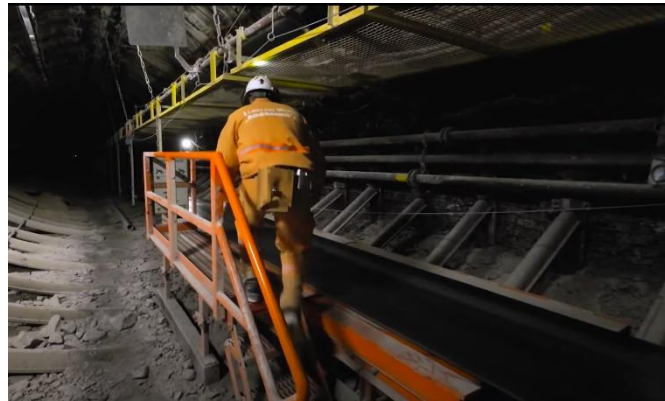
Figure 7. Underground transport means used in LW Bogdanka S.A.—Belt conveyor for transporting people. Source: photo provided by LWB.
