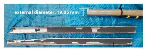
**Figure 4.** Macroscopic view of continuous scales while still in contact with a metal tube during dismantling of the SHEx in April 2019. The tube has been cut all along for the recovery of scales.
