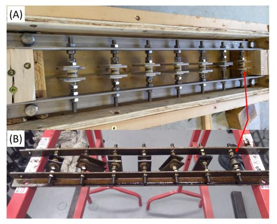
small amount of oil. The test was conducted by placing the coupons on a sample holder rack, which was placed inside a flowline at the inlet of an ORC power production unit. The sample rack before and after testing can be seen in Figure 4.
