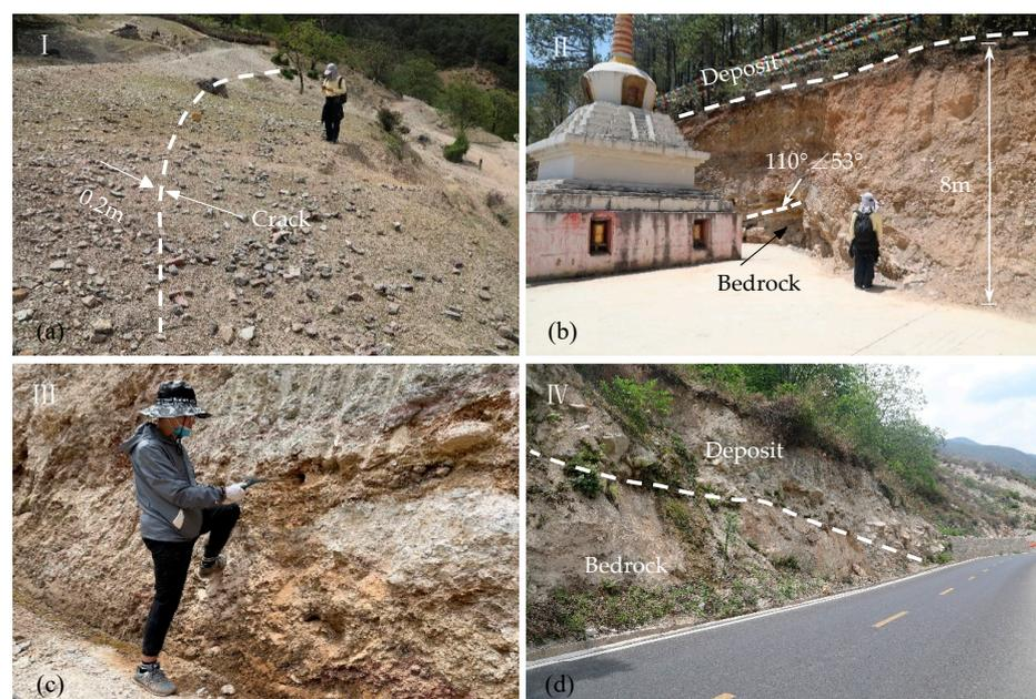
**Figure 10.** Field photos of areas I to IV. (a) The tensile crack at the trailing edge of the small landslide in area I; (b) the artificial excavation section in area II; (c) the artificial excavation section in area III; (d) bedrock outcrop at the bottom of the KZG landslide.
