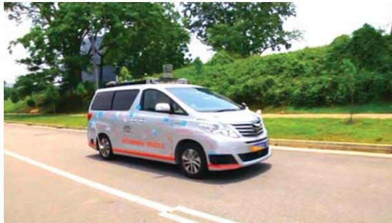
**Figure 11.** Autonomous vehicle equipped with GPS/IMU/DMI/LiDAR.
