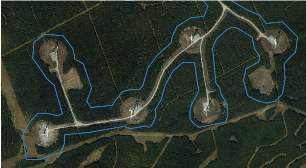
Figure 9. Land use change from coniferous forest to renewable energy (industrial or commercial units), showing the exaggeration in area caused by the mapping guidelines.
