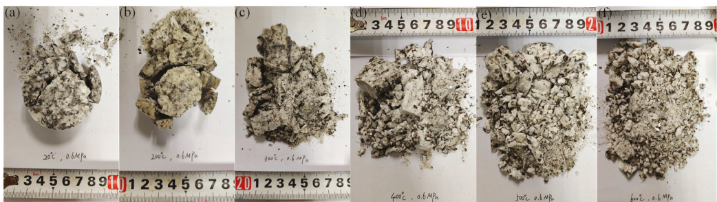
Figure 17. Relationship between fragment degree of specimens and temperature at 0.6 MPa. (a) 20 °C, (b) 200 °C, (c) 300 °C, (d) 400 °C, (e) 500 °C, (f) 600 °C.
