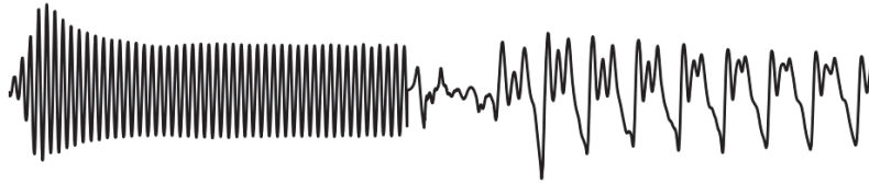
Figure 18. Example of tvconv buffer content if freezing is allowed at an arbitrary point. Old content remains in the latter part of the buffer while the first part has been written with new content.
