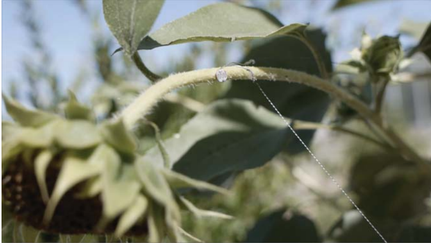
Figure 7. Sunflower embedded with photoresistor and conductive thread.
