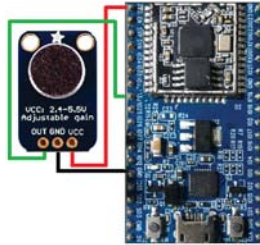
Figure 4. Wireless acoustic sensor based on ESP32 board.
