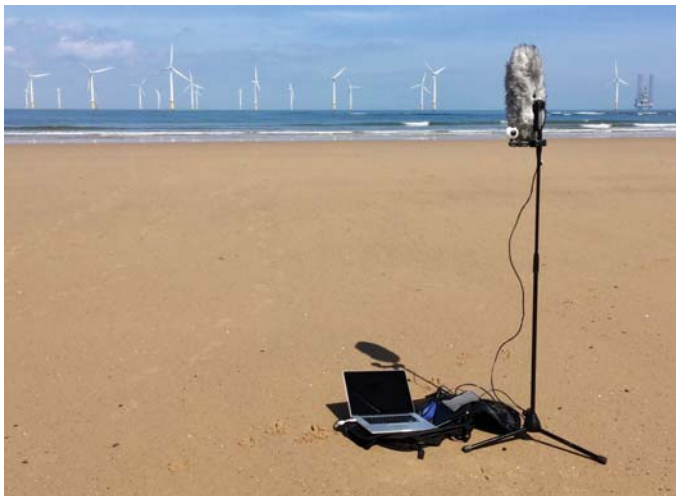
Figure 1. The setup used to record the EigenScape database: mh-Acoustics Eigenmike within a Rycote windshield, a Samsung Gear 360 camera, an Eigenmike Microphone Interface Box, and an Apple MacBook Pro. The equipment is shown here at Redcar Beach, UK: 54°37'16" N, 1°04'50" W.
