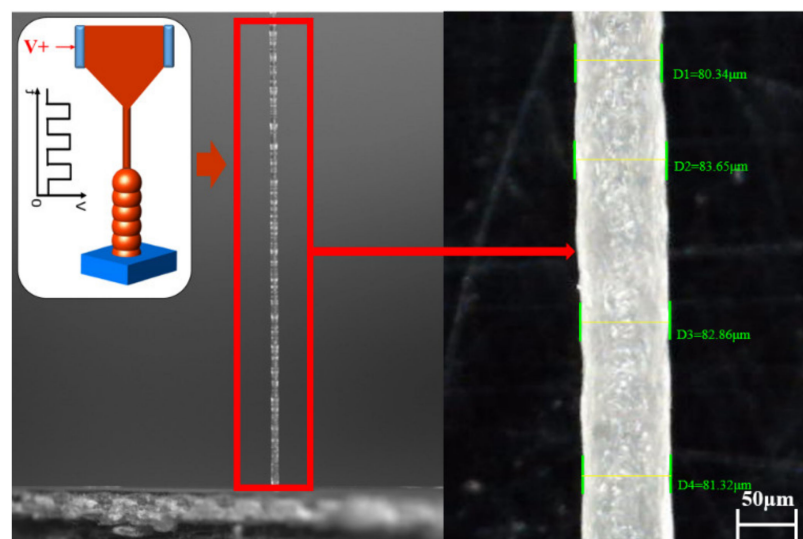
Figure 15. The deposited micro-cylinder of wax droplets with large ratio of height to diameter.
