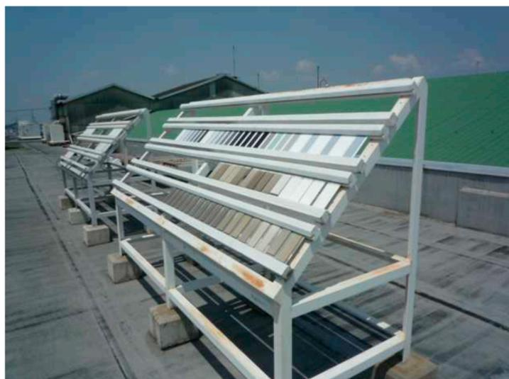
Figure 3. Outdoor exposure test at Osaka.
