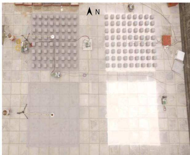
**Figure 1.** Two urban mockups and two open squares with the same size side-by-side for determining the temperature difference between pavements in urban areas and in open areas.
