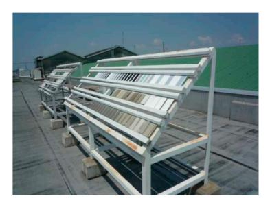
**Figure 3.** Outdoor exposure test at Osaka.
