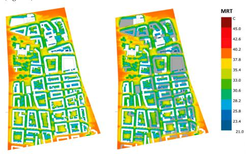
**Figure 7.** Twenty-four-hour mean radiant temperature (MRT) at street level for large-scale general densification impacts for base case (**left**) and densification scenario (**right**).
