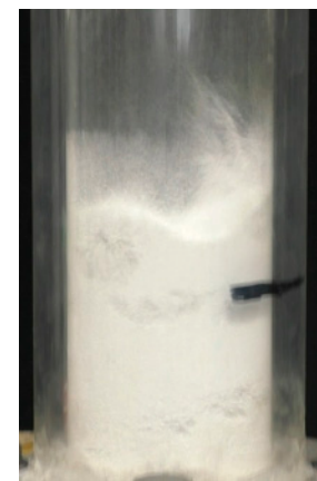
Figure 8. Classification of flow pattern and snapshots of Al_2O_3 by vertical vibrating fluidization. (a) Classification of flow pattern. (b) Fluidization bed (Region III). (c) Dispersion bed (Region IV).
