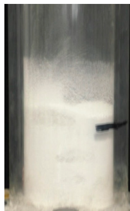
Figure 8. Classification of flow pattern and snapshots of Al_2O_3 by vertical vibrating fluidization. (a) Classification of flow pattern. (b) Fluidization bed (Region III). (c) Dispersion bed (Region IV).
