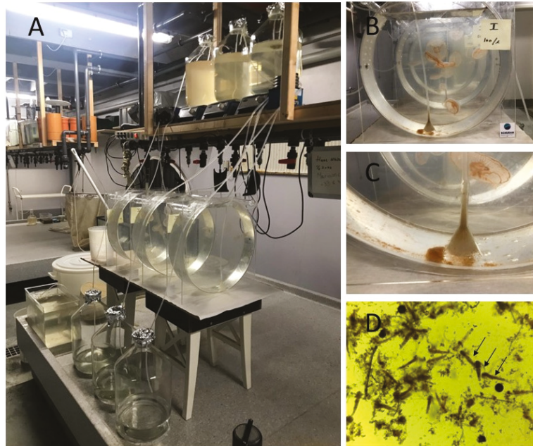
Figure 4. (A) Experimental set-up with 3 Kreislerr tanks on a bench and above that a shelf with peristaltic pumps dosing 3-day Artemia from well-mixed 10 l stock glass flasks placed on magnetic stirrers. The outflow water is collected in glass flasks below the tanks. (B) Tank with 6 small Aurelia aurita . (C) Accumulated pseudofeces on the bottom near a small glass funnel packed with cotton and connected to the opening of the outflow tube to prevent jellyfish from being sucked up. (D) Jellyfish pseudofeces consists of both living and dead 3-day Artemia (arrows) as well as black sphere-shaped unhatched cysts entangled in mucus.
