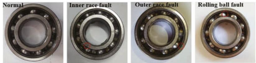
Figure 4. Different health states of rolling bearings.
