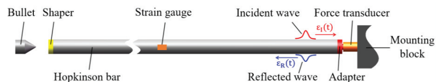
Figure 2. Schematic diagram of the principle of using Hopkinson bar to calibrate force transducer.
