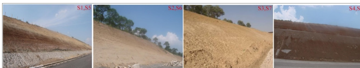
Figure 2. Filled soil in the different treatments: S1 and S5 were the weathered rock soil; S2 and S6 were the coarse silty soil; S3 and S7 were the collapsible loess; S4 and S8 were the liquefaction soil of saline soil with sandy soil.
