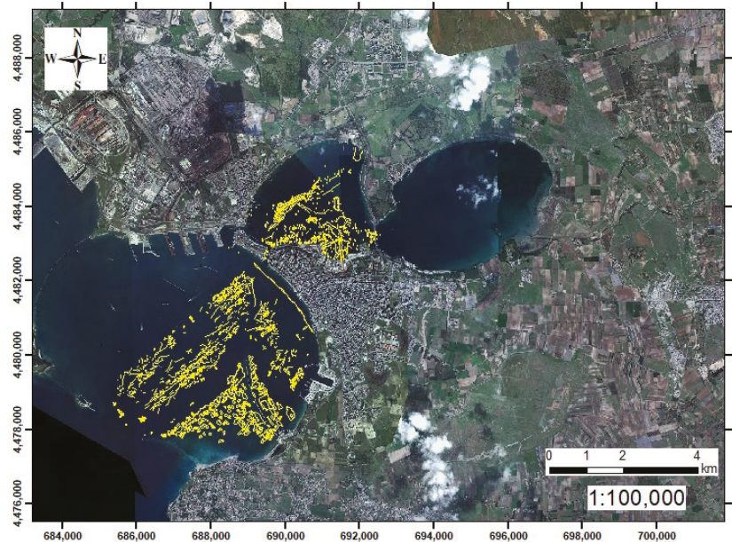
Figure 11. Distribution of anthropogenic traces detected on the seafloor of the Mar Piccolo (first Bay) and Mar Grande basins through the interpretation of SSS and MBES data.
