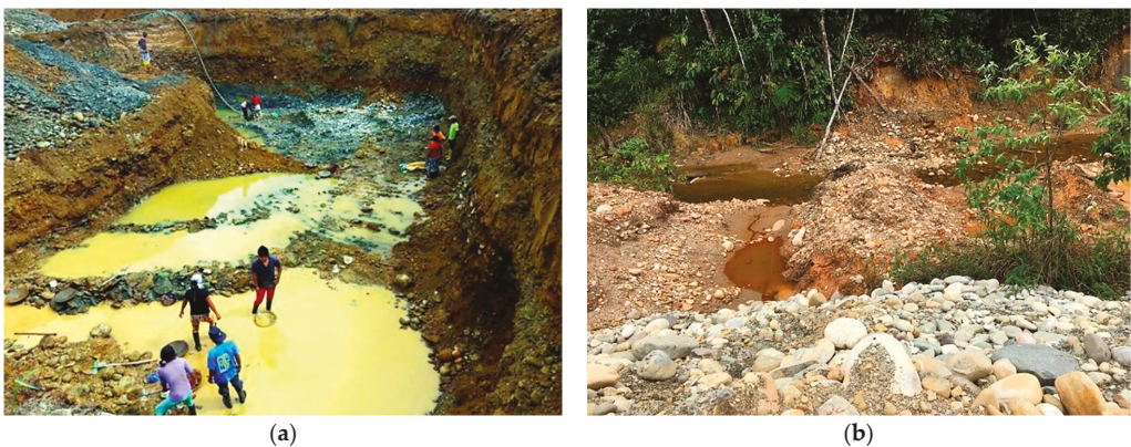
Figure 2. Gold mining impacts. (a) Pools of contaminated water exposed in the open pit; (b) debris generated by the extraction of material for gold.
