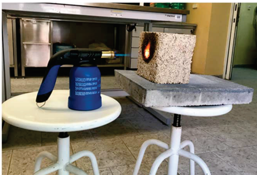
Figure 4. Hemp lime composite flame test, with the tested sample placed at a distance of 10 cm away from the flame source.
