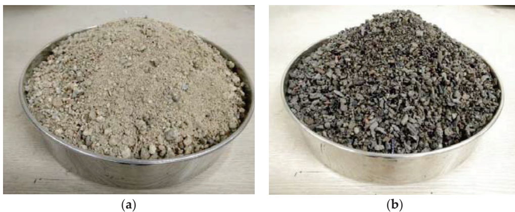
Figure 1. Crushed fine and CBA aggregates. (a) Crushed fine aggregate; (b) CBA aggregate.
