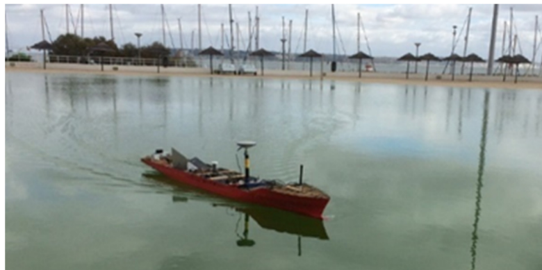
Figure 1. The free-running ship model during the manoeuvring tests.
