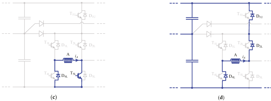
Figure 3. Topological arrangements of the multilevel converter associated to phase A in healthy condition: (a) voltage level +V_{C1} + V_{C2} ; (b) voltage level +V_{C1} ; (c) voltage level 0; (d) voltage level -V_{C1}-V_{C2} .
