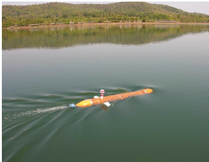
Figure 15. The MAYA AUV.
