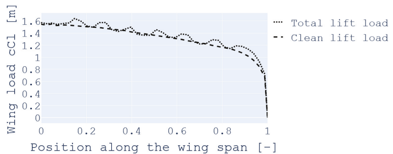
Figure 5. Lift load distribution along the dimensionless wing span.
