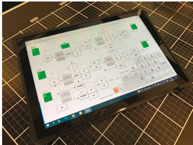
Figure 13. In-flight controller tuning application installed on the dedicated laptop.
