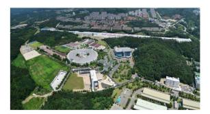
**Figure 1.** Overview of Pohang Accelerator Laboratory. The Pohang Light Source (PLS) is shown in the middle (circular building) and PAL-XFEL is shown above the PLS.
