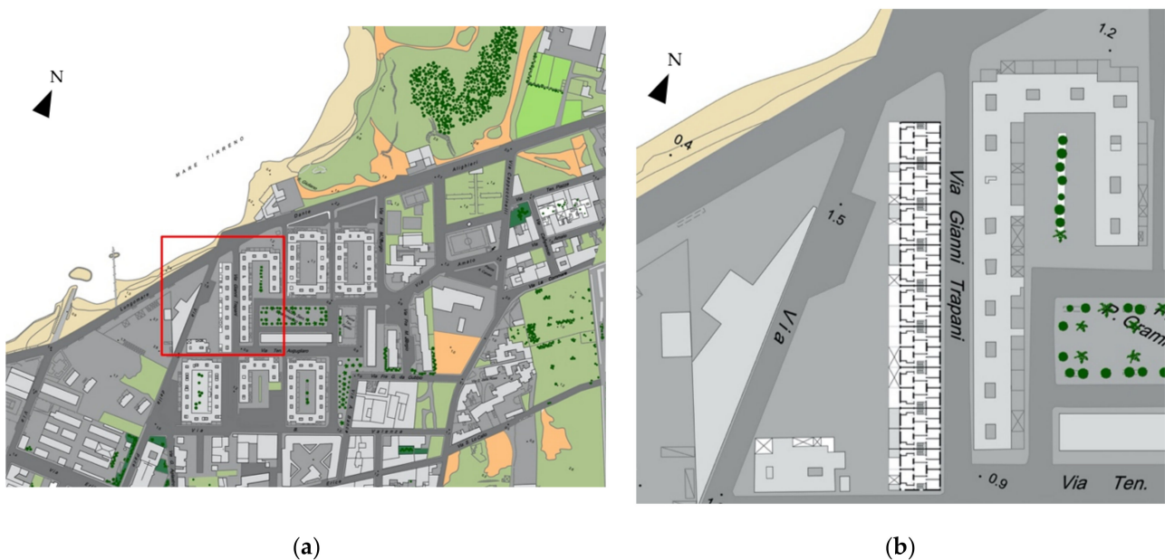
Figure 1. Plan of the Cappuccinelli District (a) and ground floor plan of the terraced block named “L” (b). Source: Rossella Corrao.
