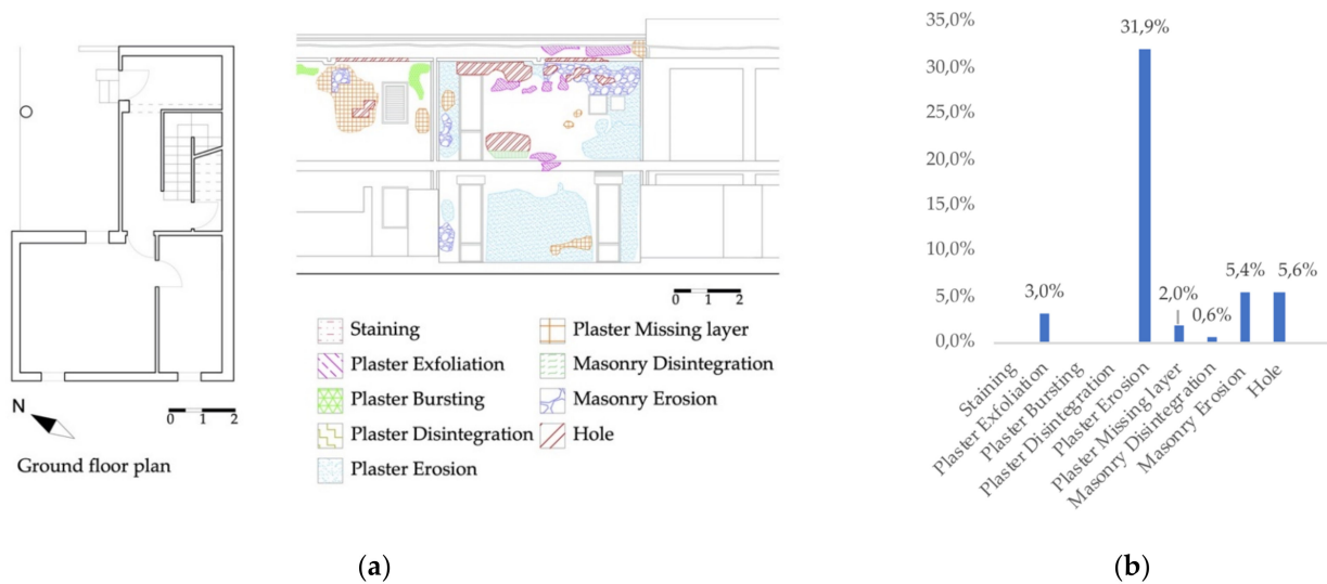
Figure 5. Ground floor plan from Valori project and representation of external visible damages on the façade (a), their extent estimated as a percentage of the analyzed façade surface (b) in the portion A (Figure 4) of the SW elevation of the “L” block. Authors: Erica La Placa, Calogero Vinci.
