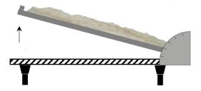
Figure 3. Scheme of the device measuring the slippery angle of repose of tested particles.
