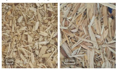
**Figure 1.** Images of wood particles: (a) microparticles (MP), (b) particles of the core layer particle-boards (PCL).
