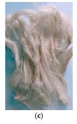
Figure 1. The materials used (a) black liquor; (b) pMDI; (c) ramie fibers.
