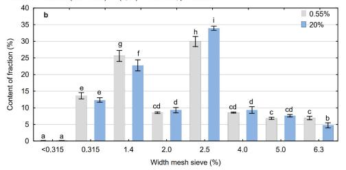
**Figure 4.** Fractional composition of microparticles (**a**) and particles of the core layer of particleboards (**b**) depending on their moisture content (a, b, c . . . —homogeneous groups as determined by the Tukey test).
