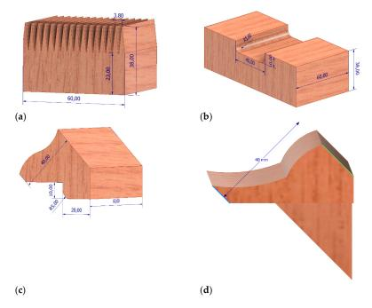
**Figure 5.** From the left: finger joint—chord of truss, UPP2 (**a**); tenon joint—chord of truss, tenon joint fragment of the lower belt UPP1 (**b**); tenon joint—diagonal member, tenon joint fragment of the crossbone UPP1 (**c**), tenon joint—diagonal member, tenon joint fragment of the crossbone UPP3 (**d**).
