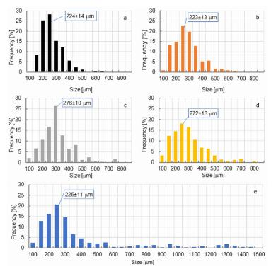
**Figure 7.** Cell size and cell size distribution of PUR foam depending on wood particle (WP) content: (a) control; (b) 5%; (c) 10%; (d) 15%; (e) 20%.
