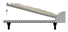
Figure 3. Scheme of the device measuring the slippery angle of repose of tested particles.
