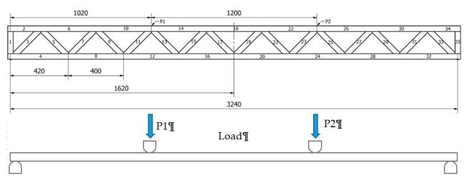
Figure 3. Truss loading diagram at two distinguished nodes ( $P_1 = P_2 = 11.12 \text{ kN}$ )—scheme B.
