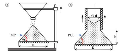
**Figure 2.** Scheme of the device measuring the angle of repose of: (**a**) microparticles, (**b**) particles of the core layer of particleboards.
