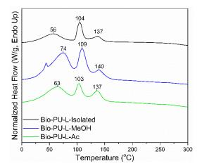
Figure 9. DSC thermograms of Bio-PU resin derived from fractionated lignin.
