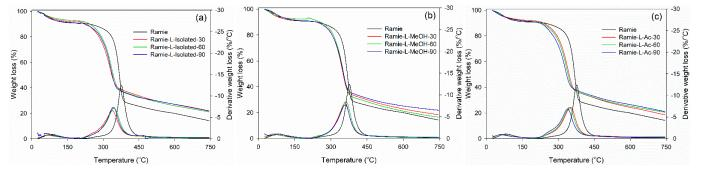
**Figure 15.** Thermal stability of impregnated ramie fibers determined with TGA-DTG: (**a**) Ramie L-Isolated, (**b**) Ramie L-MeOH, and (**c**) Ramie L-Ac.
