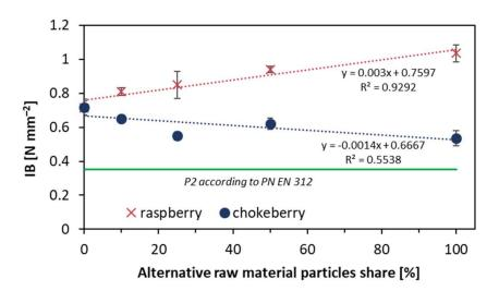
Figure 7. Internal bond of the tested composites.
