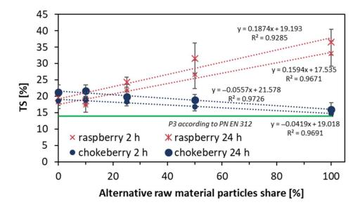
Figure 8. Thickness swelling of the tested composites.
