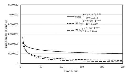
Figure 4. Particle mass in purified air for narrow surfaces treatment line.
