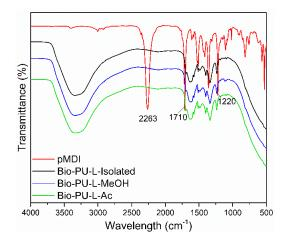
Figure 8. ATR-FTIR spectra of Bio-PU resin derived from fractionated lignin.
