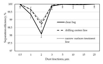
**Figure 6.** Fractional separation efficiency for 272 days of operation time of filter bags in individual dust extraction installations.
