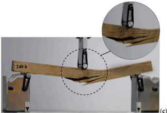
**Figure 5.** The fracture plane of the weathered oak wood at three exposure times: 24 h (**a**), 150 h (**b**), and 240 h (**c**) under the static bending test.
