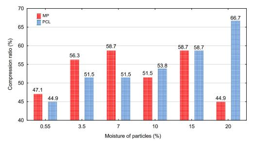
Figure 6. The compression ratio of wood particles depending on their moisture content.
