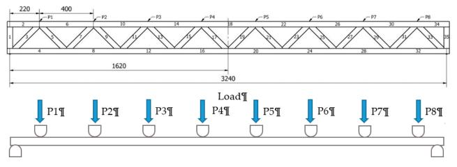
Figure 2. Truss loading scheme at each node ( $P_i = P = 2.78 \text{ kN}$ )—scheme A.
