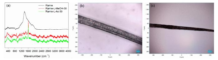
**Figure 12.** Micro Confocal Raman analysis of ramie fiber: (**a**) Typical Raman spectra of ramie fiber, (**b**) image of ramie fiber before impregnation at  $10 \times$  magnification, and (**c**) image of ramie fiber after impregnation at  $10 \times$  magnification.
