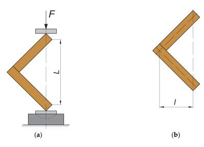
**Figure 6.** Test procedure. Reprinted with permission from Ref. [11]. 2021 BISMAR. (**a**) Type of loading of the tested samples; (**b**) determination of the bending arm.
