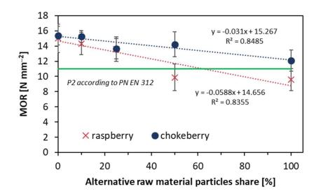
Figure 5. Modulus of rupture of the tested composites.
