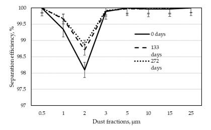
**Figure 8.** Fractional separation efficiency for filter bags from the dust extraction installation of a narrow surfaces treatment line in particular periods of use.
