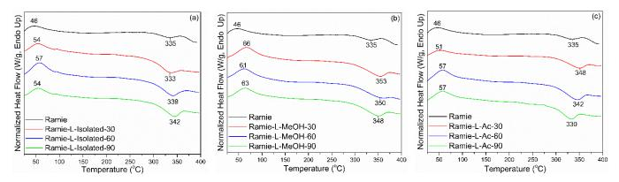
Figure 14. DSC analysis of impregnated ramie fibers: (a) Ramie L-Isolated, (b) Ramie L-MeOH, and (c) Ramie L-Ac.
