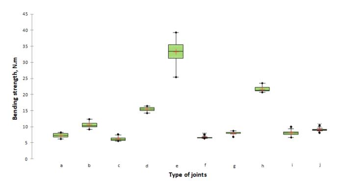
**Figure 8.** Bending strength under the compression test of L-type corner joints made of lightweight panels. The letter index of the type of joints is according to Figure 4.
