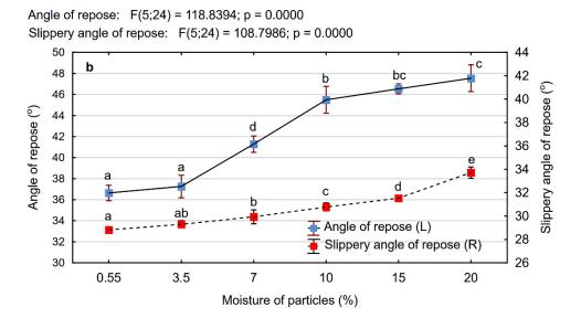
**Figure 7.** The angle of repose and the slippery angle of repose of microparticles (**a**) and particles of the core layer of particleboard (**b**) depending on their moisture content (**a**, **b**, **c** . . . —homogeneous groups as determined by the Tukey test).
