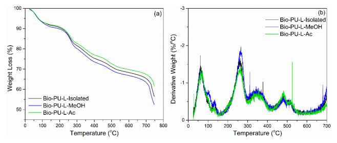
Figure 10. Thermal degradation of Bio-PU resin derived from lignin: (a) TGA, (b) DTG.
