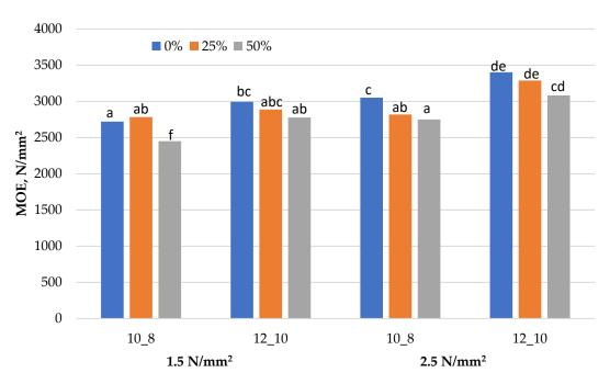
Figure 2. Modulus of elasticity (MOE) of particleboards produced.
