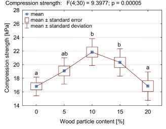
**Figure 11.** Compression strength of PUR-WP composition depending on wood particle content. Different letters indicate homogeneous groups of mean values determined by one-factor ANOVA with Tukey's test.
