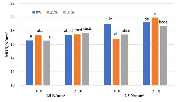
Figure 1. Bending strength (MOR) of particleboards produced.
