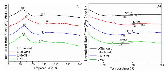
Figure 4. DSC thermograms of lignin before and after fractionation: (a) full thermogram, (b) enlarged thermogram.
