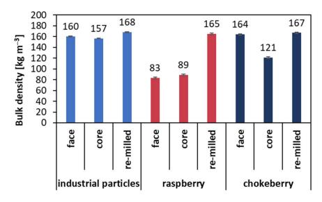
**Figure 4.** Bulk density of particles used to produce composites, considering the particles produced by the re-milling of composites.
