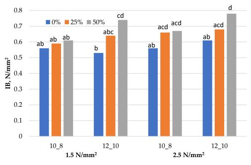
Figure 3. Internal bond (IB) of particleboards produced.
