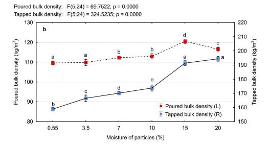
**Figure 5.** Poured bulk density and the tapped bulk density of microparticles (**a**) and wood particles of the core layer of particleboard (**b**) depending on their moisture content (a, b, c . . . —homogeneous groups as determined by the Tukey test).
