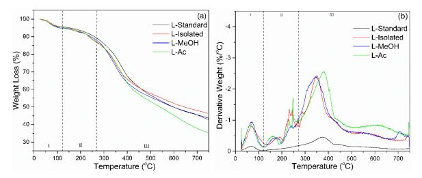
Figure 5. Thermal behavior of lignin before and after fractionation: (a) TGA, (b) DTG.
