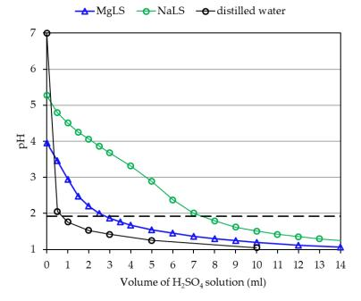
**Figure 5.** Curves of variation of pH as a function of titration with  $0.309 \text{ M H}_2\text{SO}_4$  of lignosulfonate solutions or distilled water. Mass of the solution is 40 g. Concentration of lignosulfonate is 6%. The dotted line shows the pH of the cured resin with  $(NH_4)_2\text{SO}_4$  without lignosulfonates.
