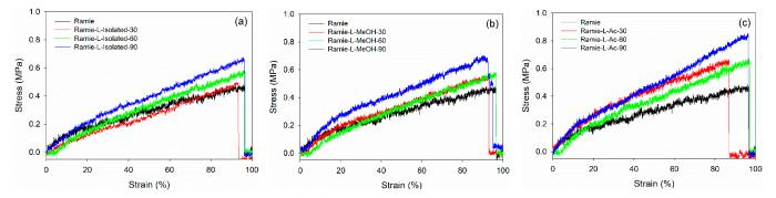
**Figure 16.** Typical stress–strain curve of ramie fibers before and after impregnation: (**a**) Ramie L-Isolated, (**b**) Ramie L-MeOH, and (**c**) Ramie L-Ac.
