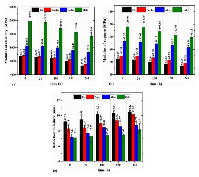
Figure 3. The variation of MOE (a), MOR (b), and deflection to failure (c) in weathered wood samples.
