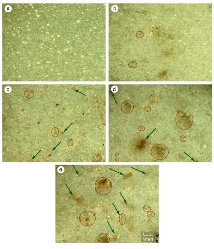
**Figure 8.** Light microscope photos of PUR samples with addition of different amount of WP: (a) control; (b) 5%; (c) 10%; (d) 15%; (e) 20% (green arrow—wood particles; red circle—structure disorders, large pores). All scale bars of figures are the same.
