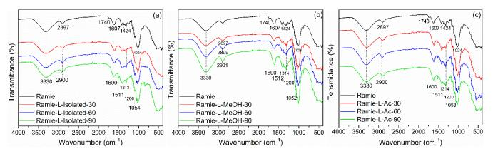
Figure 11. FTIR Spectra of impregnated ramie fibers: (a) Ramie L-Isolated, (b) Ramie L-MeOH, and (c) Ramie L-Ac.
