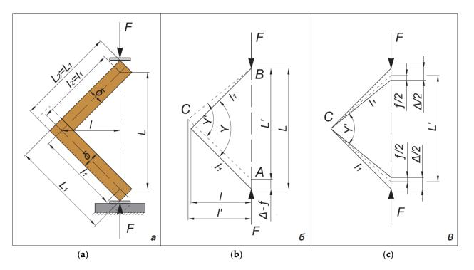
**Figure 7.** Test scheme and deformation under arm compression bending load of the test samples of end corner joints made of lightweight panels. Reprinted with permission from Ref. [11]. 2021 BISMAR. (a) Type of loading and dimensions of the tested samples; (b,c) scheme of loading and determination of the deformation of the tested samples.
