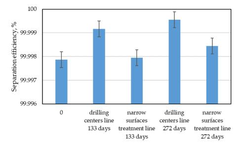
Figure 9. Total separation efficiency for all installations.
