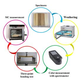
Figure 1. The experimental procedure employed in this study.
