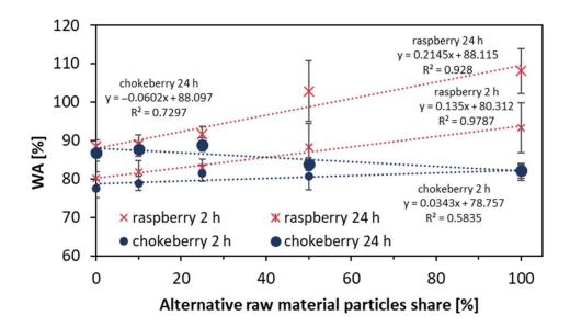
Figure 9. Water absorption of the tested composites.
