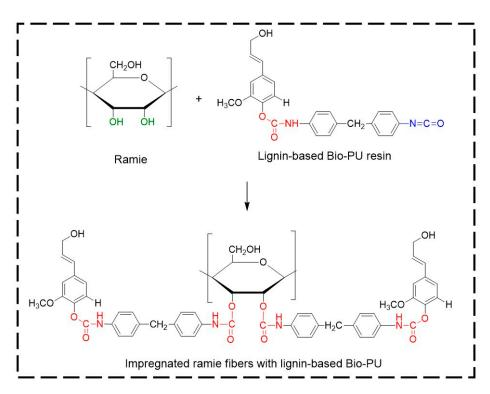
Figure 13. The possible scheme reaction of ramie fibers with lignin-based Bio-PU resin.
