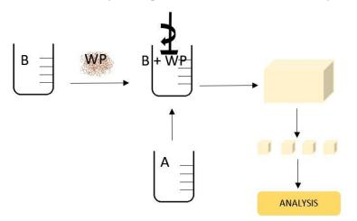
Figure 3. Scheme of PUR manufacturing (A-polyol; B-isocyanate; WP-wood particles).
