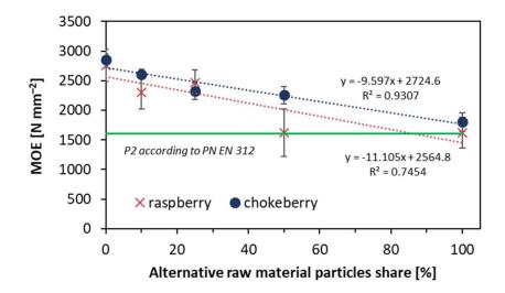
Figure 6. Modulus of elasticity of the tested composites.
