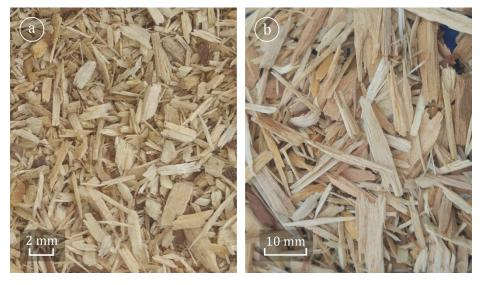
**Figure 1.** Images of wood particles: (**a**) microparticles (MP), (**b**) particles of the core layer particleboards (PCL).
