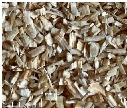
Figure 1. Wood particles used as a filler for PUR foams.
