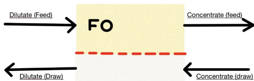
Figure 6. Forward osmosis process principle.
