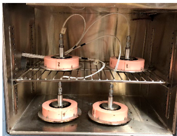
(a) Asphalt Binder Cracking Device (ABCD) test apparatus
