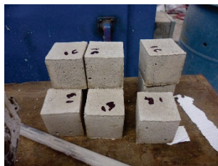
(a) Compression test probes: 0.05 × 0.05 × 0.05 m
