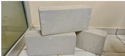
(c) Produced cellular concrete blocks: 0.12 × 0.2 × 0.4 m
