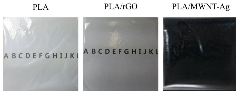
Figure 3. Transparency of PLA, PLA/rGO 1.0 wt%, and PLA/MWNT-Ag 1.0 wt% films.
