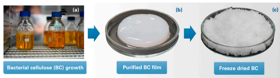
Figure 1. BC growing (a) a purified BC hydrogel (b) and BC after shredding and freeze drying (c).
