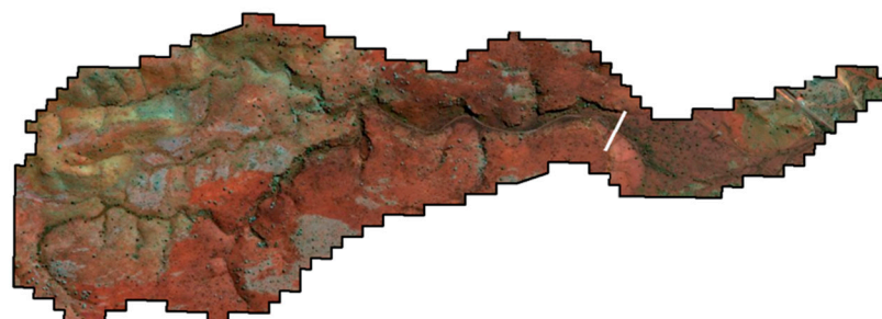
Figure 7. Catchment with a digitized white line showing a cross section (Plot output) for the TUFLOW model.
