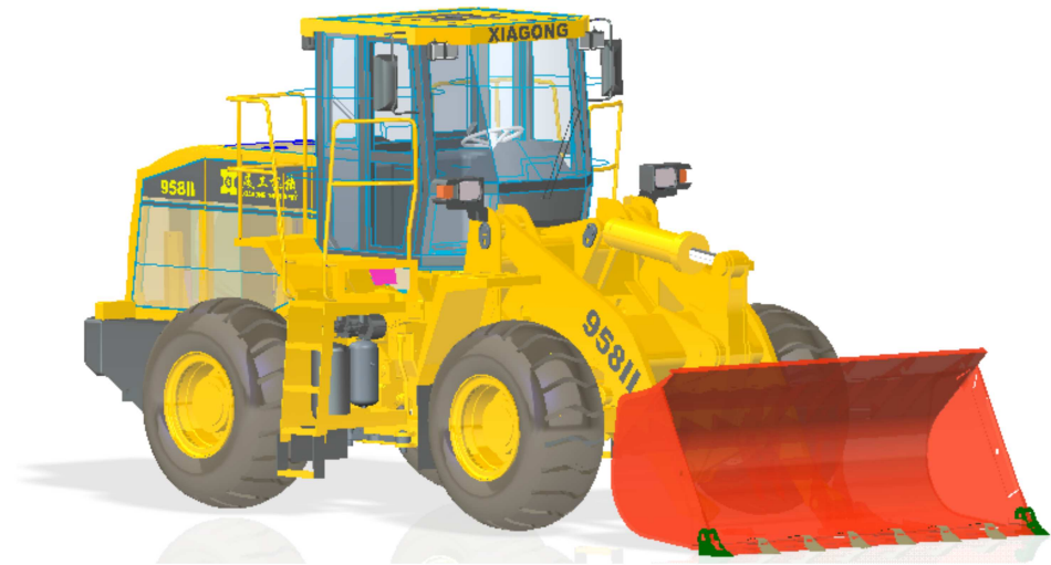
Figure 3. The three-dimensional model of the 958 N loader.
