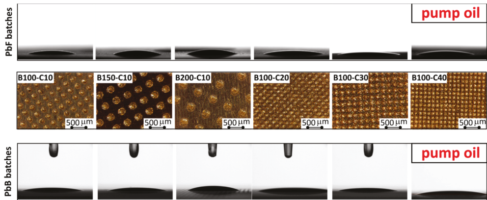
Figure 8. Oil droplets for all Pb-based and Pb-free textured surfaces.
