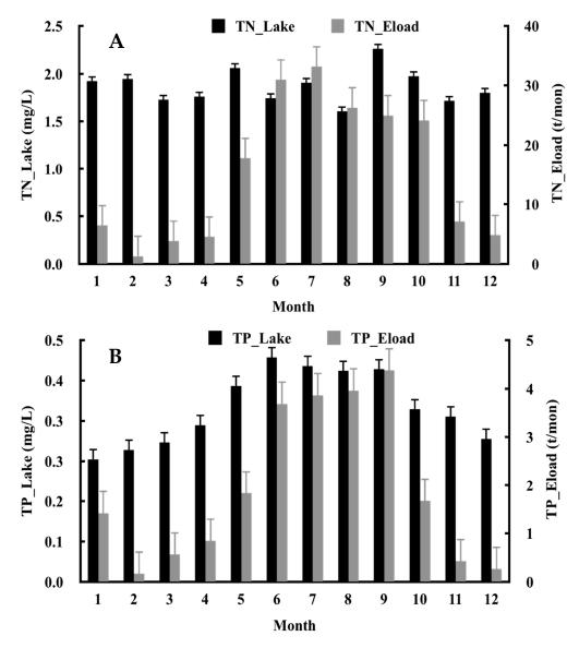
**Figure 5.** Mean monthly concentrations of lake TN (TN\_Lake) with positive standard errors (black), and tributary loadings of TN (TN\_Eload) with positive standard errors represented (grey) for January 2010–April 2018 (**A**). Mean monthly concentrations of lake TP (TP\_Lake) with positive standard errors (black), and tributary loadings of TP (TP\_Eload) with positive standard errors represented (grey) (**B**) for January 2010–April 2018.
