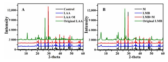
**Figure 4.** (**A**) statistical XRD patterns of control, LAA, LAA+M, and Original LAA. (**B**) statistical XRD patterns of M, LMB, LMB+M, and Original LMB. Original LAA and Original LMB are substances that are not mixed with sediments respectively.
