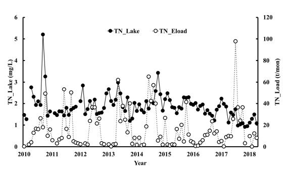
**Figure 3.** Monthly lake TN concentration (TN\_Lake), represented by black solid circles and solid line (left *Y* axis), and total tributary TN inputs (TN\_Eload) represented by black hollow circles and dash line (right *Y* axis), during January 2010–April 2018.
