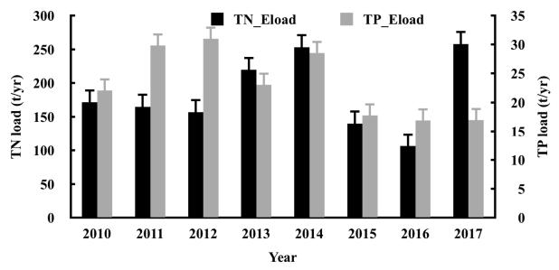
**Figure 6.** Annual tributary external loadings of TN (TN\_Eload) with positive standard errors (black, left *Y* axis), and TP (TP\_Eload) with positive standard errors (grey, right *Y* axis), in Lake Xingyun for 2010–2017.
