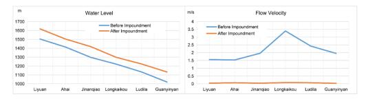
**Figure 6.** Changes in water level in front of dams and velocity in reservoirs after cascade hydropower development on the middle reaches of the Jinsha River.
